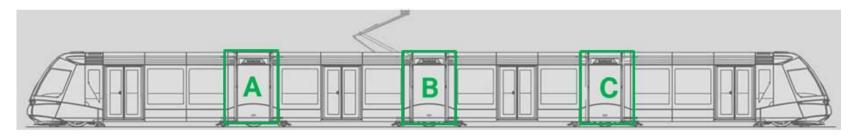
Dimensions of usable spaces: 206x225cm for each space (A – B - C, on both the sides), also considering an application divided in three segments, of the following dimensions:
